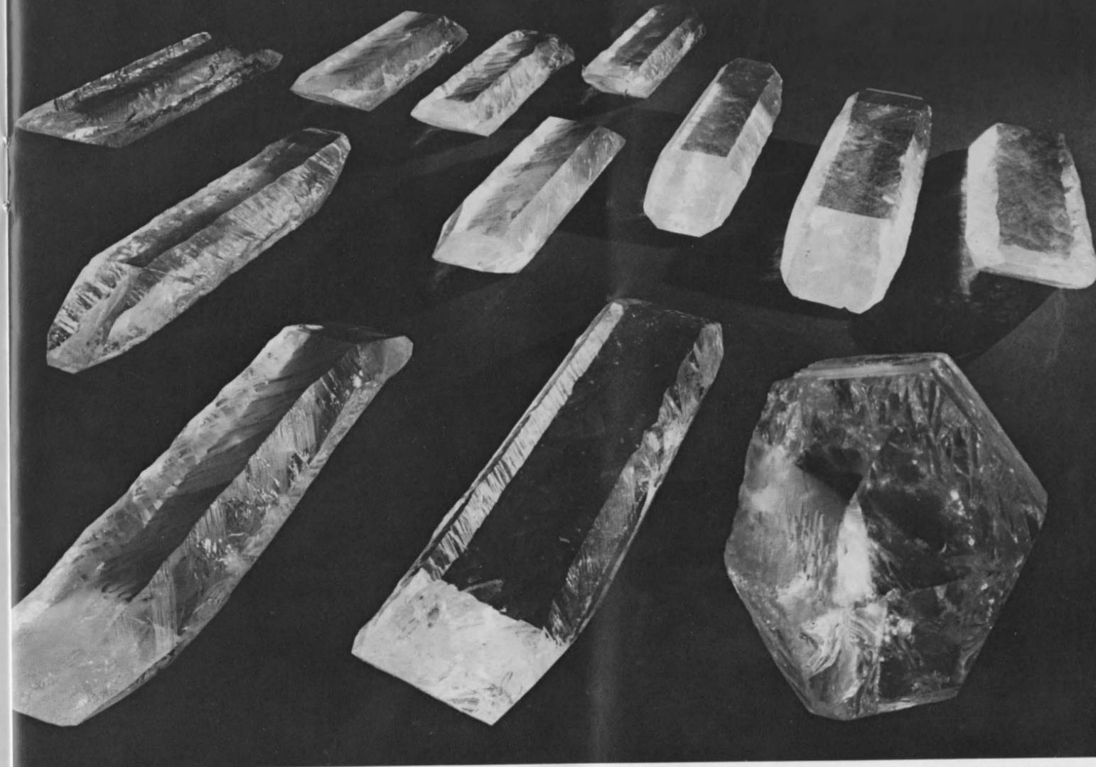
*Top Left:* A new, man-made crystal, lithium tantalate, is grown at WE's Merrimack Valley facility north of Boston as the first practical alternative to quartz for use in communications transmission equipment.
