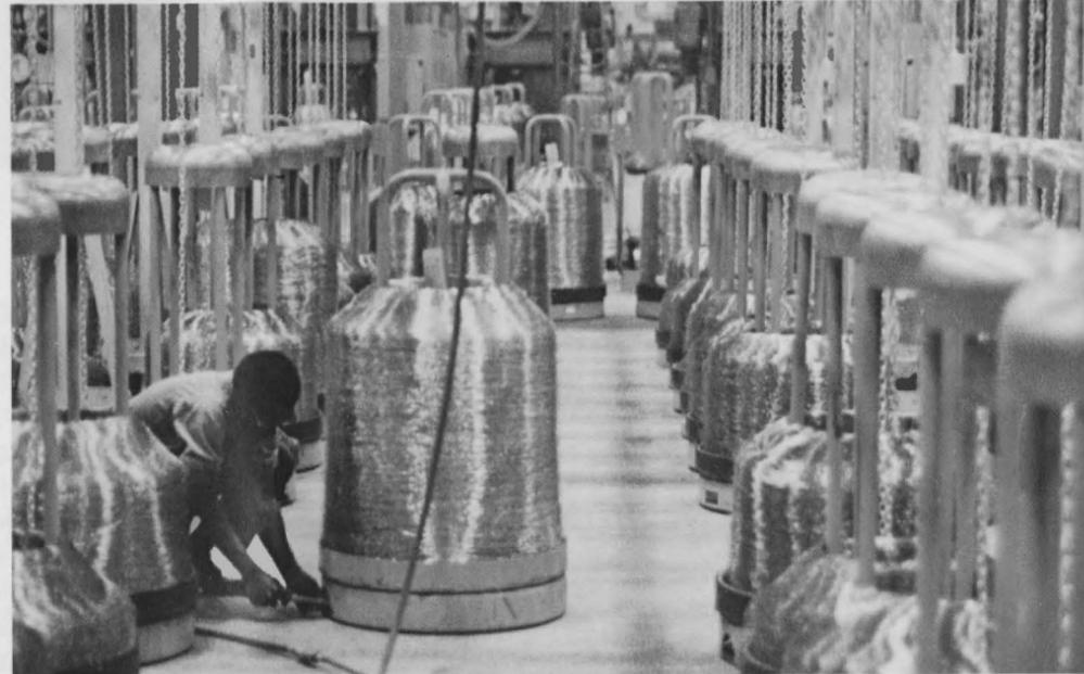
*Bottom Left:* These spools of copper wire being prepared for pulp insulating at Atlanta are moved on a cushion of air because of their weight. The wire will later be made into exchange pulp cable and used to connect central offices.
