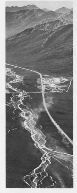
**Rivers & Streams** The pipeline crosses more than 800 streams and roughly parallels the floodplain channels of 5 large rivers. Most stream and floodplain crossings are constructed in the conventional above-ground or buried modes. In 13 crossings, however, the pipe will be supported on bridge structures.
