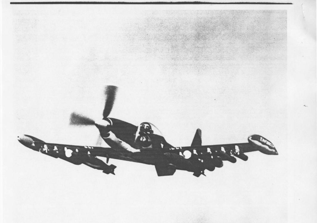
ENFORCER with 10 underwing weapons pylons and six internal 50 salibar mashing
