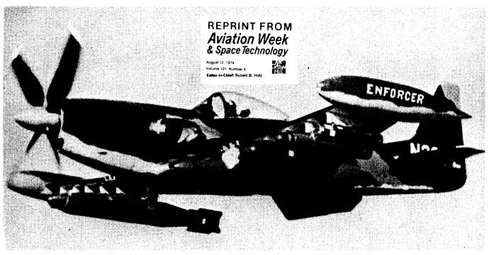
Cavailer/Piper Enforcer close-support aircraft, which would be produced by Lockheed-Georgia under an option, carries a mix of weapons on its 10 ordnance stations. Note the large over-the-wing exhaust port for the Avco Lycoming T55-L-9 gas turbine engine. The small residual thrust exhausted provides a low infrared signature for heat-seeking missiles. Muzzles of six .50-cal. guns are barely visible in the wings.
