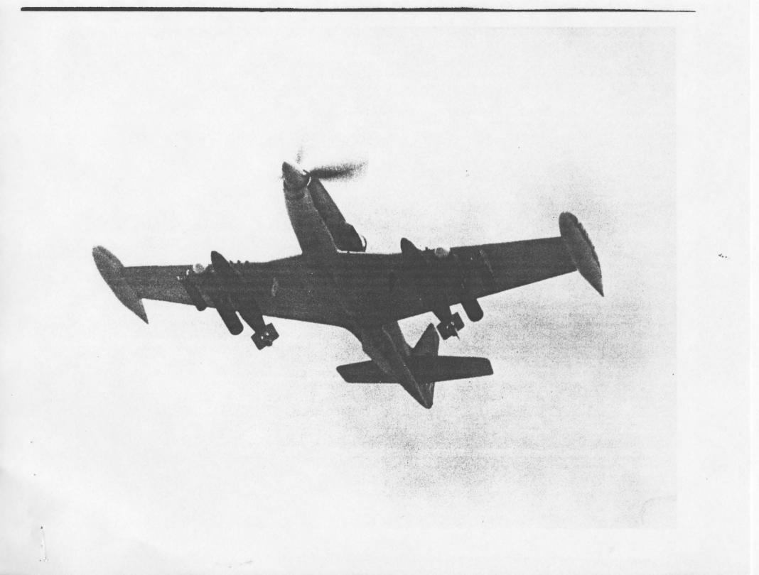
This gun camera photo, taken during live ordnance weapons testing, shows the ENFORCER carrying two 1000 lb. finned fire bombs, two 16-round flare dispensers, and two 7-round rocket launchers, with the muzzles of its six internally mounted machine guns protruding from the leading edge of the wing. Additionally, 2000 rounds of cal. 50 ammunition are carried. (No. 1)
