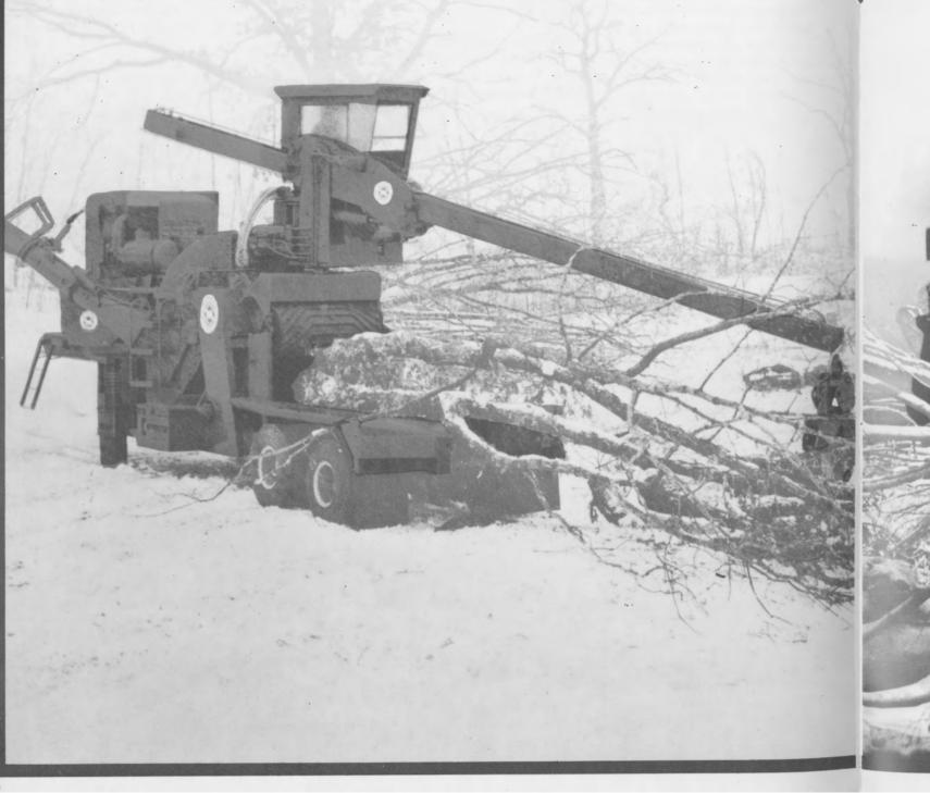
With four models offered, there is a *Chiparvestor* to meet every terrain condition, size of forest and chip production requirement. The *30/72* Model *Chiparvestor* accomodates whole trees up to 30 inches by 72 inches in diameter (no tree grows perfectly round). Other *Chiparvestor* model numbers— 18/32, 14/28 and 10/18 –describe the size tree each model *Chiparvestor* will handle. Price, weight and size descend from the Model 30/72 to the 10/18.
