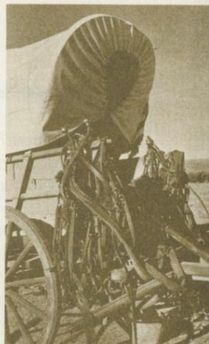
four feet shorter and weigh about 1500 pounds. All have five-foot wheels on the rear, four-foot wheels on the front for easier turning.
