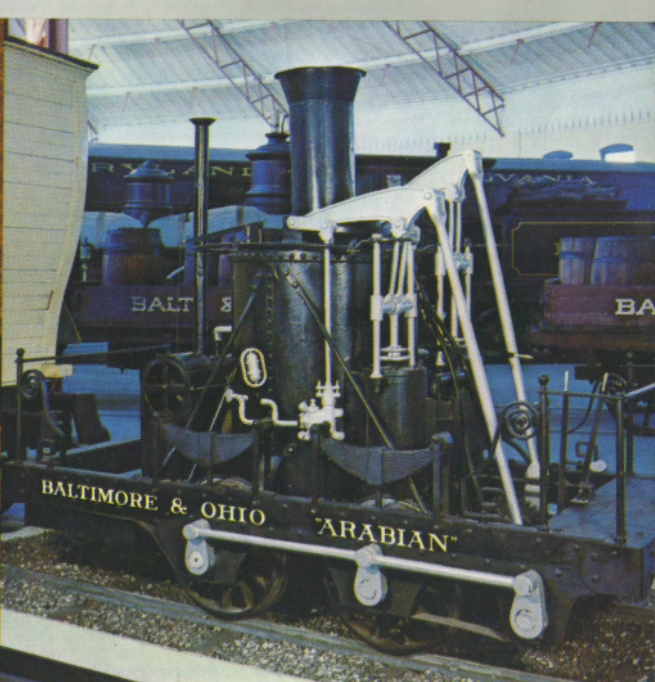
The Arabian (model), an 1834 grasshopper-type locomotive, was the first steam engine to make it up the grade, unassisted, at Parr's Spring Ridge near Mt. Airy, Md., ending plans for proposed cable hoists to lift cars.
