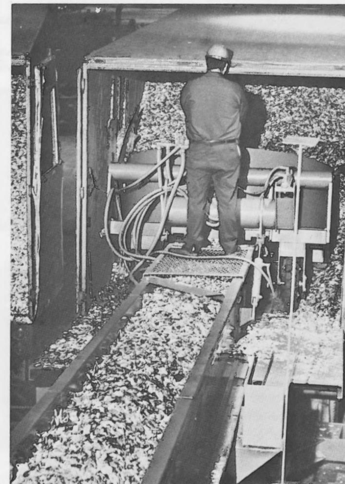
Morbark Chip Scoop enters a van of chips and unloads the van in approximately 10 minutes. Chips are conveyed directly to the central drum screen.
