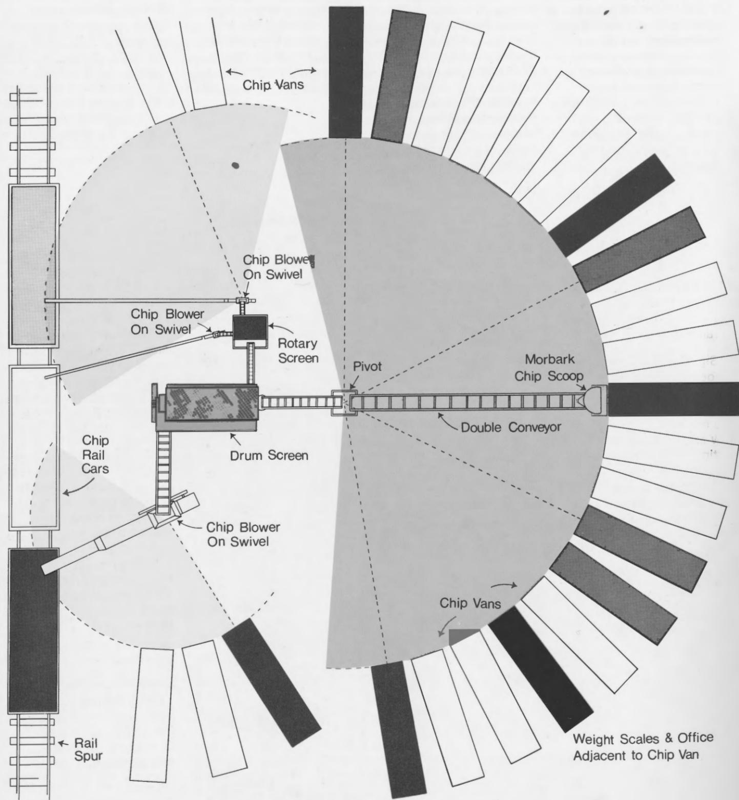
Nowhere in the world has there been a dimensional wood chip processing system capable of unloading, sorting and reloading 200 tons of wood chips per hour. Morbark's new *Class-A-Fiber System* can accomplish that feat routinely 24 hours a day.
