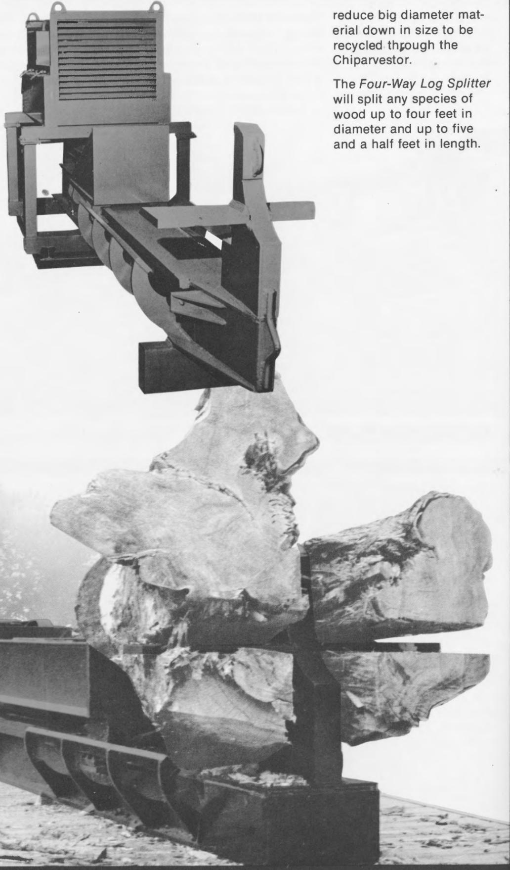
reduce big diameter material down in size to be recycled through the Chiparvestor.
