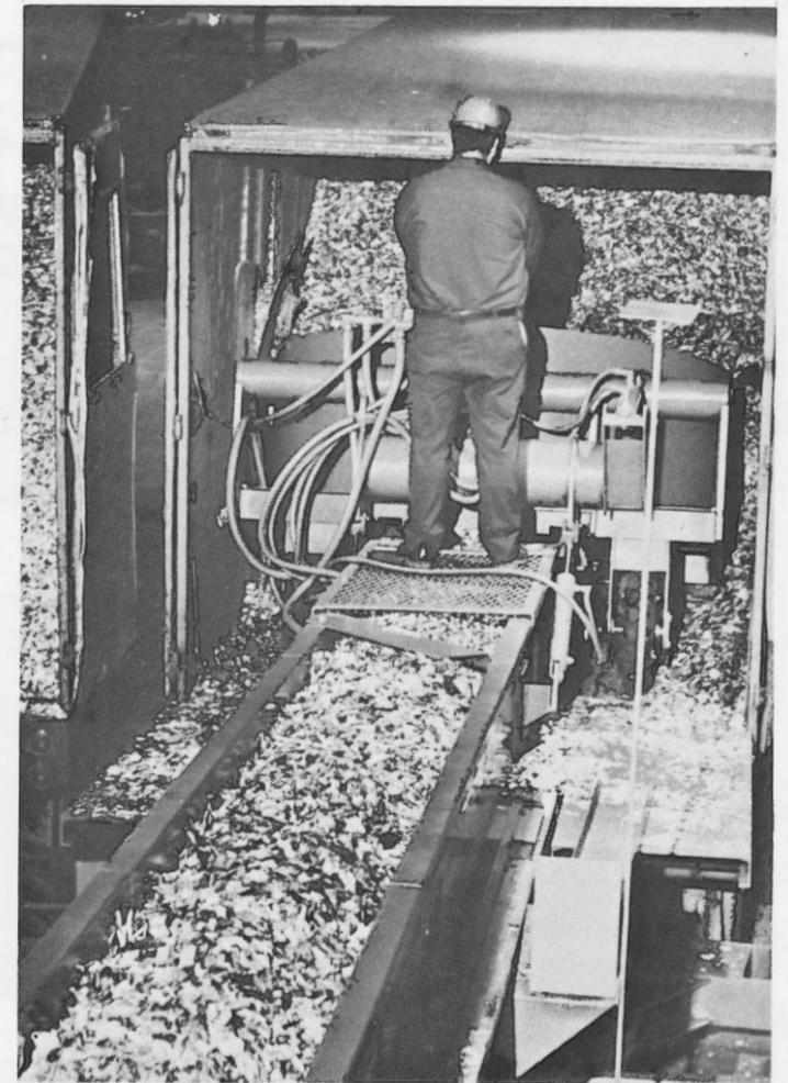
Morbark Chip Scoop enters a van of chips and unloads the van in approximately 10 minutes. Chips are conveyed directly to the central drum screen.
