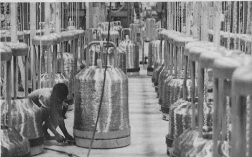
Top Left: This aluminum wire is used in the manufacture of aluminum cable. WE has been a leader in this development.
