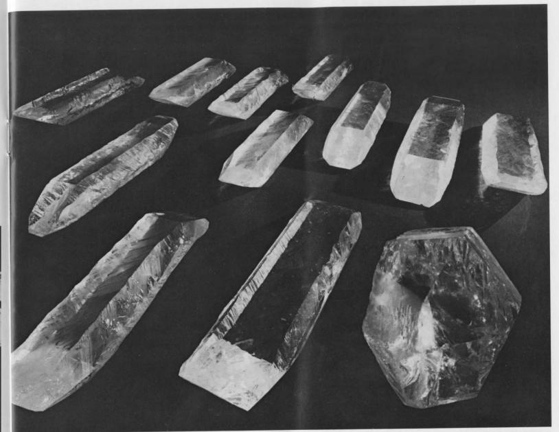
Top Left: A new, man-made crystal, lithium tantalate, is grown at WE's Merrimack Valley facility north of Boston as the first practical alternative to quartz for use in communications transmission equipment.
